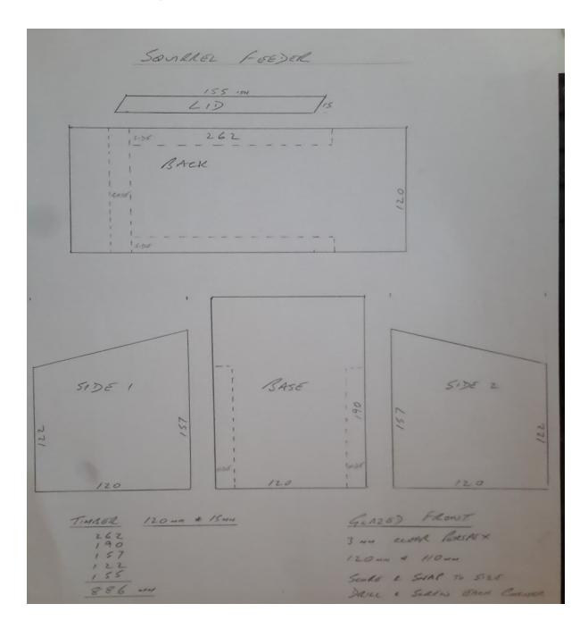
Alternative glazing option is to route a groove inside the sides at the front and slide the perspex in.
